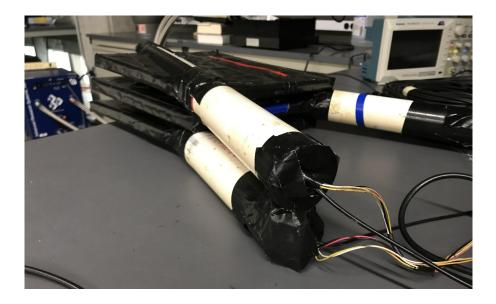
This setup can show if and how flux is affected by external factors (air pressure, temperature, et cetera). Coincidences: 1-fold, 2-fold, 3-fold
