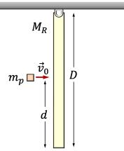
A. What is the moment of inertia of the "rod + particle" system about the suspension point after the collision?
